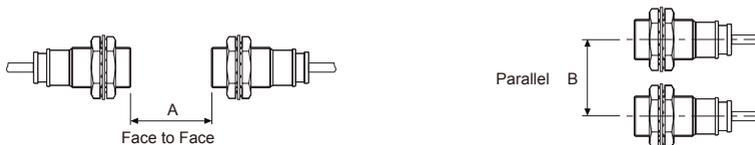
When sensors are mounted on metallic panel, it is required to protect the sensors from being affected by any metallic object except target. Therefore, be sure to provide a minimum distance as below chart indicates.
